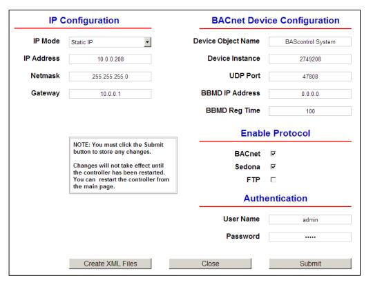
The System Configuration page allows for IP and BACnet device configuration. Select the desired protocol(s) from this page.
