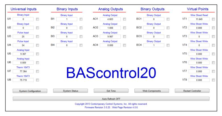
The main web page provides an overview of the 20 real IO points plus the eight virtual points. Access to other configuration pages is possible through the main page. Point forcing is possible.
