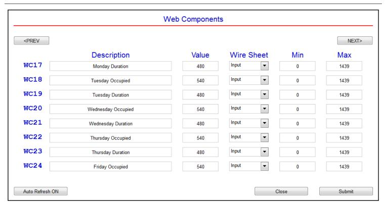
Up to 48 web components are available for data exchange between web pages and wire sheets without the need of a programming tool. These components are used for scheduling.
