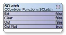
Set/Clear Latch – single-bit level-triggered single-bit data storage
