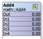
Four-input addition — results in the addition of four floats.
