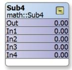
Subtract four — results in the subtraction of four floats.
