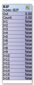
Binary to float encoder — 16-bit binary to float conversion.
