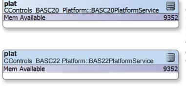
The BAScontrol20/22 platform kit has only one component that advises the programmer how much usable memory is available for application programming. It is recommended that the usable memory not fall below 8,192 bytes. It can be found in the services folder and can be copied onto the wire sheet. The output type of this component is a *Long*.
