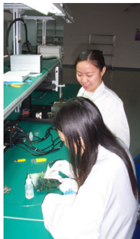
Workers in Contemporary Controls’ Suzhou facility do finishing touches at printed circuit board assembly. The company manufactures its products in Downers Grove, Illinois, Suzhou, China and Eisleben, Germany.
