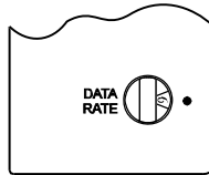
Data rate switch set to the default position 6 (2.5 Mbps).
