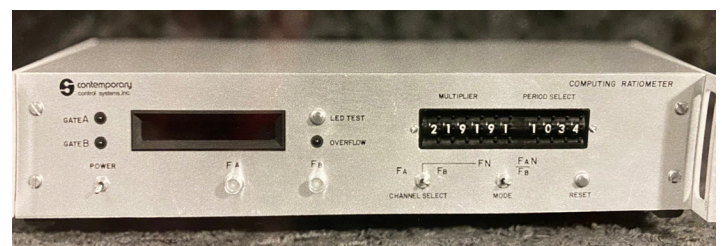
The first- microprocessor-based computing ratiometer, developed by Contemporary Controls in 1975.
