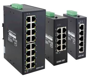
The EISW series consists of 5, 8 and 16-port 10/100 Mbps Ethernet switches that can be DIN-rail mounted in control panels and powered from a NEC class 2 limited energy power source. The EISW switches are UL Listed as Information and Communication Technology Equipment under safety standard UL 62368-1 and can be installed in a UL 508A panels without invalidating the control panel listing.
